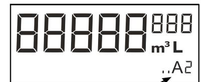
The figure after the 'A' states how many times the meter has been adjusted. In a completely new meter both of these characters will be out.
